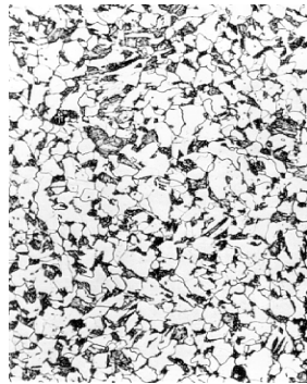
25 mm Plate ASTM No. 12.3
