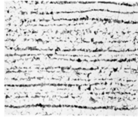
Figure 15 The Effect of Microstructural Banding on HIC and SSC Test Performance of A516-60
