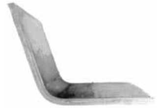
Figure 3: 3/8" thick ArcelorMittal USA HARDWEAR 450F formed with 3T bend radius parallel to the rolling direction
